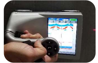
GPR shows position of rebar in concrete bridge abutment
